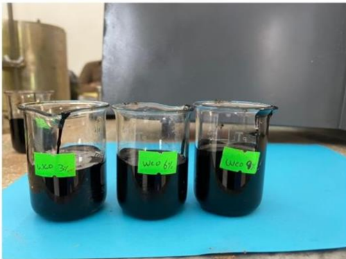
Figure 4. Mixing of WEO in bitumen
