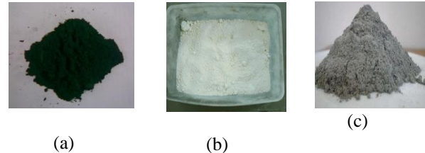
Figure 1. The physical appearance of materials (a) Bagasse ash (b) Metakaolin (c) Fly ash
