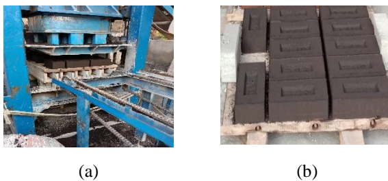
Figure 3. Brick production at an industrial scale
