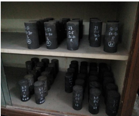
Figure 2. Ambient curing of the prepared specimens.
