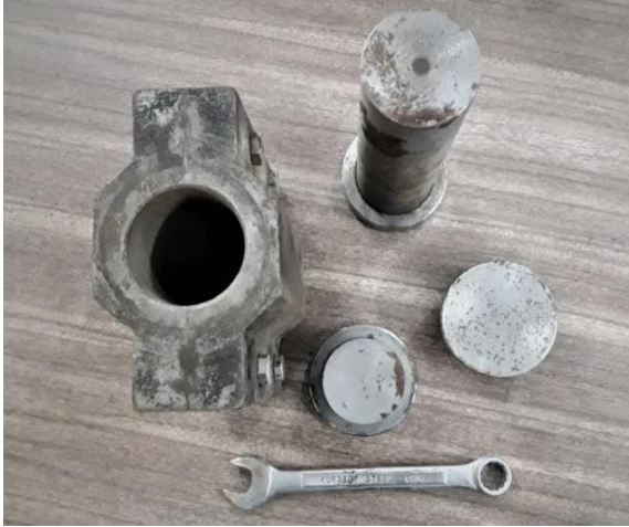
Figure 1. Set up for casting the cylindrical specimens.
