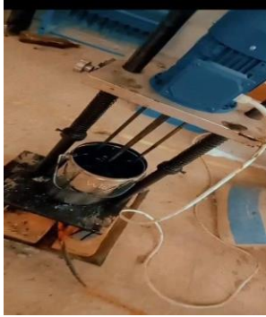
Figure 4. Mixing of WEO in bitumen
